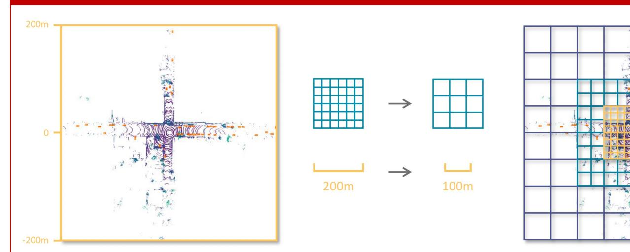
Existing 3D LiDAR detectors struggle to detect far away objects (e.g. 300m) due to time and compute constraints.
